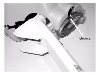
Figure 27: Feed horn groove
